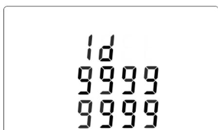
From the setup menu, use **P** and **MD/HZ** buttons to select extended address option.
