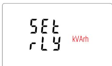
Use **P** and **MD/PF/HZ** buttons to choose kWh or kvarh.
