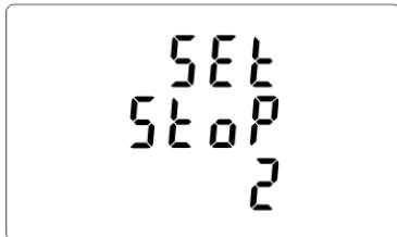
From the set up menu, use **P** and **MD/PF/HZ** buttons to select the stop bit option.
