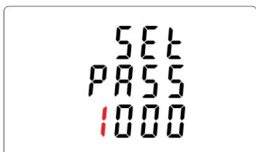
Press and hold **E** to enter the change password routine. The new password screen will appear with the first digit flashing.
