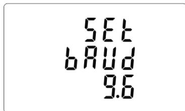
From the set up menu, use **P▼** and **MD/PF/HZ▲** buttons to select the Baud rate option.
