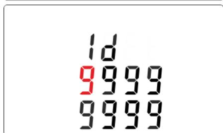
Press **E** button to enter the selection routine. The current setting will be flashing.
