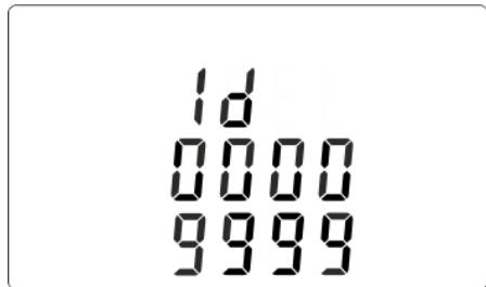
Use **P** and **MD/HZ** buttons to change digits and **E** to change position, to choose Modbus address (00000000 to 99999999).
