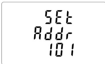
Use **P** and **MD/HZ** to change digits and **E** to change position, to choose Modbus address (001 to 250).
