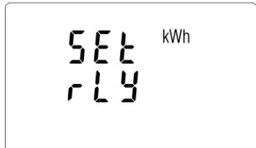
From the setup menu, use **P** and **MD/PF/HZ** buttons to select the pulse output option.
